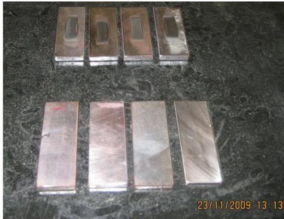
Figure 1. Standard test specimen of size 75mmX26mmX6mm
